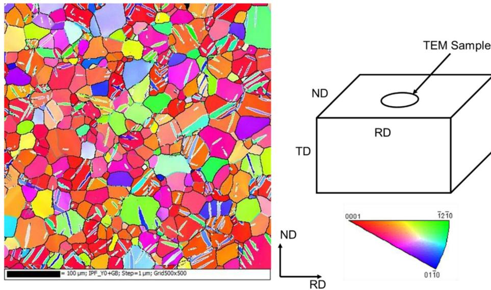
Fig. 1. A typical electron backscatter diffraction (EBSD) inverse pole figure (IPF) image of Mg-3wt.%Y alloy, which is deformed in compression along the RD. The schematic shows the macroscopic sample directions of the alloy in relation to the transmission electron microscope (TEM) foil preparation. Here RD, TD and ND refer to rolling, transverse and normal directions, respectively.
