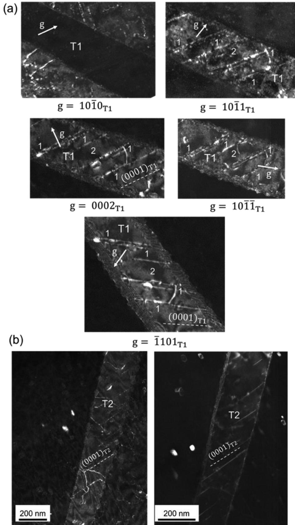
Fig. 8. (a) WBDF micrographs showing the variation in dislocation contrast in the domain of twin T1 for the various operating reflections. (b) The TEM images showing stacking fault contrast parallel to the trace of the basal plane after tilting the sample about the  $[\bar{1}010]$  axis of twin T2.
