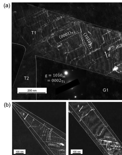
Fig. 7. WBDF TEM images showing the structure of dislocations inside twin T1. (a) The dislocations are visible for  $g = 0002$  reflection, suggesting that they have a strong  $\langle c \rangle$  component, and the dislocations are projected in different directions on the plane of the micrograph. (b) Shows there are a few non-basal  $\langle c \rangle$  components inside T1 for  $g = 10\bar{1}0$ . The solid lines in the micrographs represent the twin boundary.
