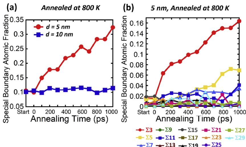
Fig. 12. (a) Special boundary fraction for both grain sizes as a function of annealing time at 800 K. (b) A detailed breakdown of each special  $\Sigma$  type for the  $d = 5 \text{ nm}$  sample, showing that  $\Sigma 3$  boundaries exhibit the fastest increase while  $\Sigma 5$ ,  $\Sigma 7$ , and  $\Sigma 11$  interfaces also become more common.
