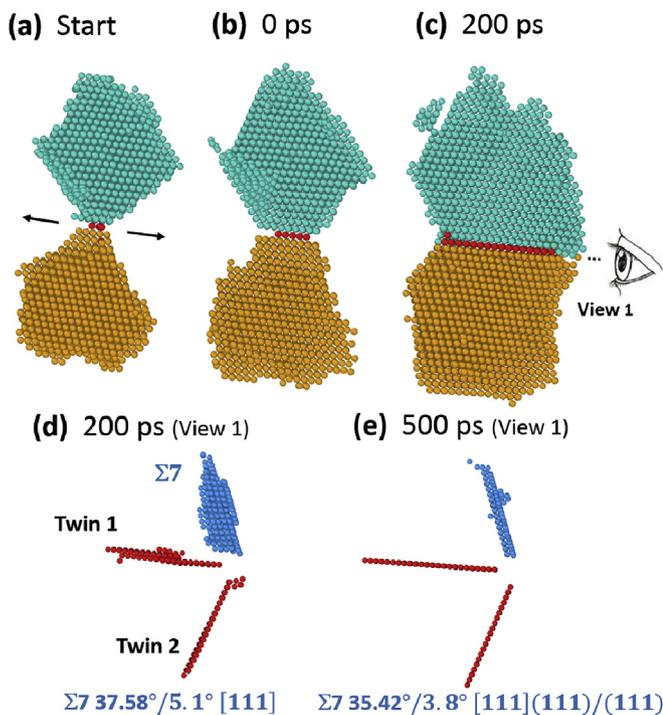
Fig. 13. (a)–(c) Curvature-driven grain boundary migration leads to  $\Sigma 3$  boundary lengthening in the  $d = 5 \text{ nm}$  sample during annealing. Additional evidence of grain boundary facet removal is shown in (d) and (e), where a well-defined (111) plane forms along the  $\Sigma 7$  boundary after 500 ps of annealing.
