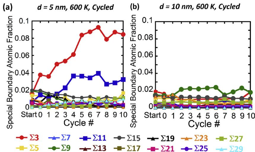
**Fig. 7.** Special boundary fraction for the (a)  $d = 5$  nm at 600 K sample shows an increase in  $\Sigma 3$  and  $\Sigma 5$  boundary content. (b) The  $d = 10$  nm samples experience very little evolution of the special boundary fraction during cycling.
