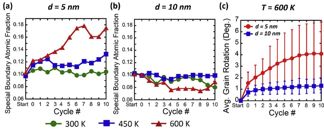
**Fig. 6.** Special boundary fraction of mechanically cycled samples for (a)  $d = 5$  nm and (b)  $d = 10$  nm for all testing temperatures. (c) Average grain rotation, measured as the disorientation from a grain's starting configuration, for 5 nm and 10 nm average grain sizes cyclically loaded at 600 K.
