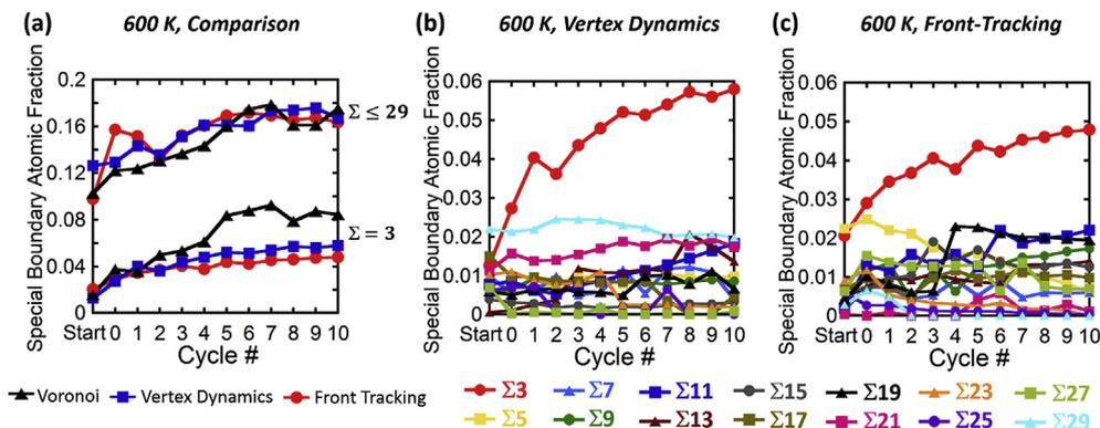
**Fig. 11.** (a) The upper curves show the special boundary fraction evolution for all boundaries with  $\Sigma \leq 29$  as a function of cycle number. The lower curves compare the difference in  $\Sigma 3$  evolution for all three starting configurations. Detailed evolution of special boundary fraction for all special  $\Sigma$  types is shown as a function of cycle number for the (b) Vertex Dynamics and (c) Front-Tracking samples, respectively.
