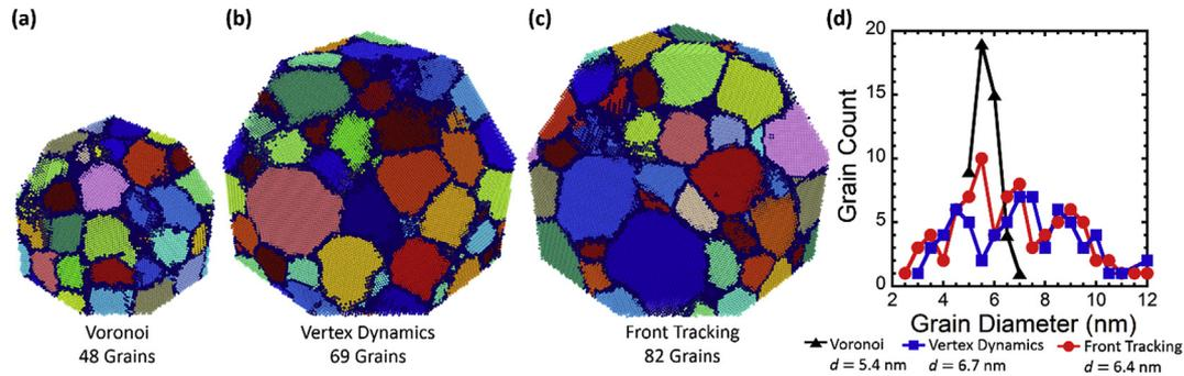
**Fig. 10.** (a)–(c) Visual comparison of the three different starting configurations post annealing at 600 K with grains colored according to GTA identification. (d) The grain size distribution for all three samples before cycling was performed showing a much narrower distribution for the Voronoi sample. Calculated average grain size for each sample are also listed below the figure.
