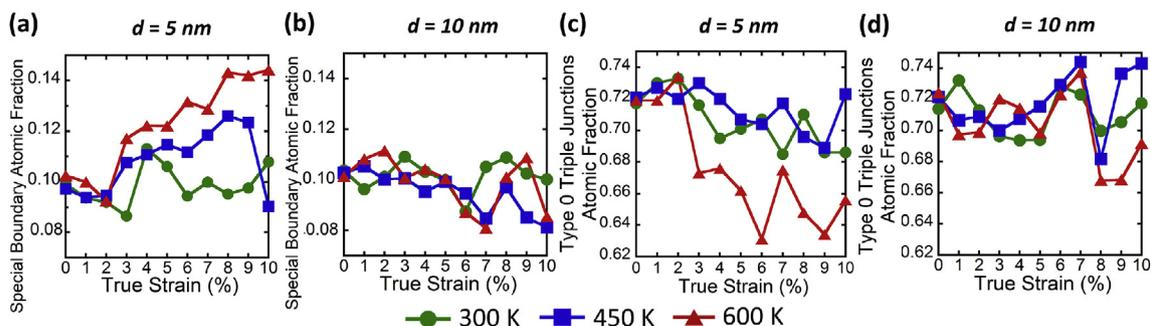
**Fig. 4.** The evolution of special boundary fraction for (a)  $d = 5$  nm and (b)  $d = 10$  nm monotonic tension tests at all testing temperatures. (c) Type 0 triple junction analysis for  $d = 5$  nm sample, showing evolution which was inversely proportional to the special boundary fraction evolution. (d) Type 0 triple junction fraction for the  $d = 10$  nm grain size exhibits fluctuations, but no discernable upward or downward trend.
