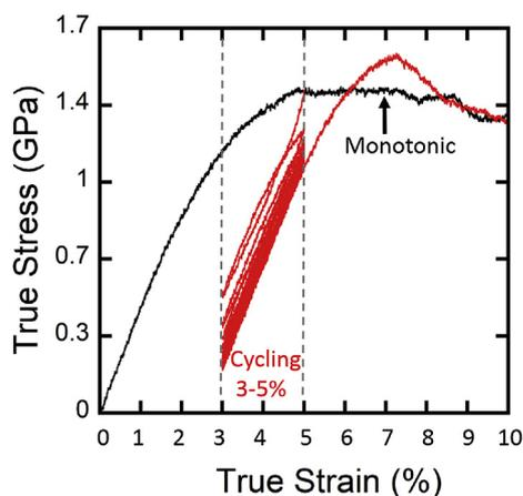
**Fig. 1.** Mechanical response of  $d = 5 \text{ nm}$  sample loaded monotonically (black line) and cyclically (red line) at 300 K. Dotted grey lines illustrate the mechanical cycling procedure. Identical loading procedures were performed at 450 K and 600 K. (For interpretation of the references to colour in this figure legend, the reader is referred to the web version of this article.)
