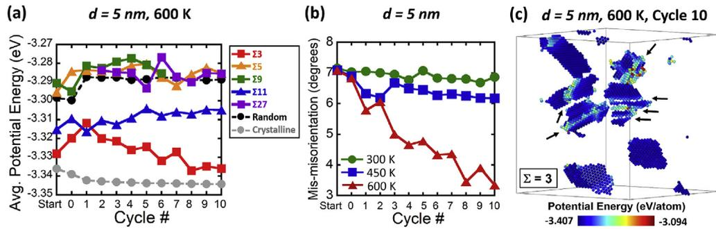
**Fig. 8.** (a) Average potential energies of select special boundary atoms, random boundary atoms, and crystalline atoms during cycling. (b) Mis-misorientation of  $\Sigma 3$  boundaries as a function of cycle number. (c)  $\Sigma 3$  boundaries at Cycle 10, with black arrows indicating facet steps which allowed coherent segments to form.
